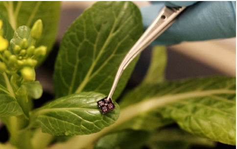
A tiny smart chip with sensors can be placed on plants like choy sum to monitor plant growth and health in real-time.
