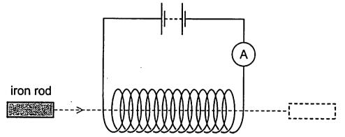
An iron rod is passed through the solenoid at constant speed. Which graph shows the variation with time t of the reading I of the ammeter?
