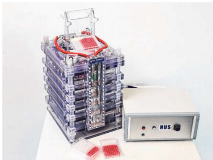
A bioreactor (above) passes the magnetic fields through the cells. A 10-minute exposure can cause cells to multiply better and survive longer than the outcome of adding animal serum to cells, says Prof Franco-Obregon.
