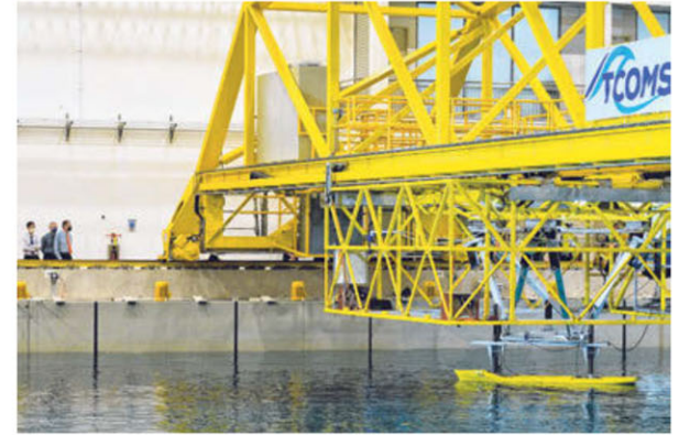
A mini vessel (left) being used to track movement of the waves, and the towing carriage (right) of the ocean basin facility. Tcoms said that the basin's capacity to generate waves and undercurrents allows it to mimic conditions in shallow, intermediate and deep waters. ST PHOTOS: NG SOR LUAN
