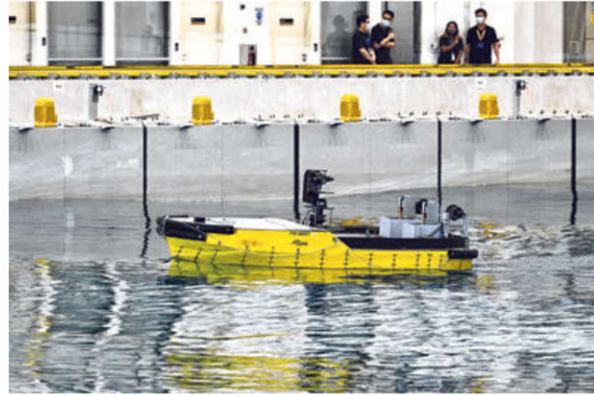
A mini vessel (left) being used to track movement of the waves, and the towing carriage (right) of the ocean basin facility. Tcoms said that the basin's capacity to generate waves and undercurrents allows it to mimic conditions in shallow, intermediate and deep waters. ST PHOTOS: NG SOR LUAN
