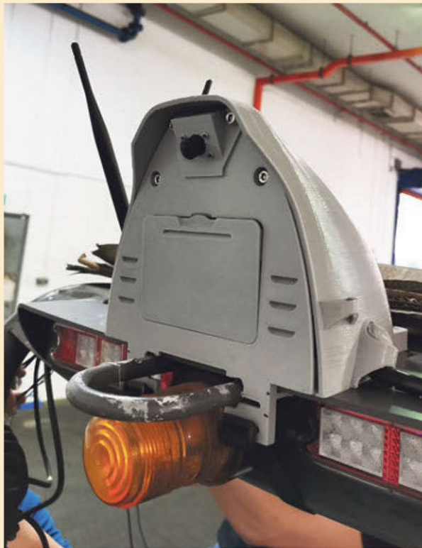
Keppel Logistics developed Scaped to alert forklift drivers of potential obstacles. PHOTO: KEPPEL LOGISTICS
