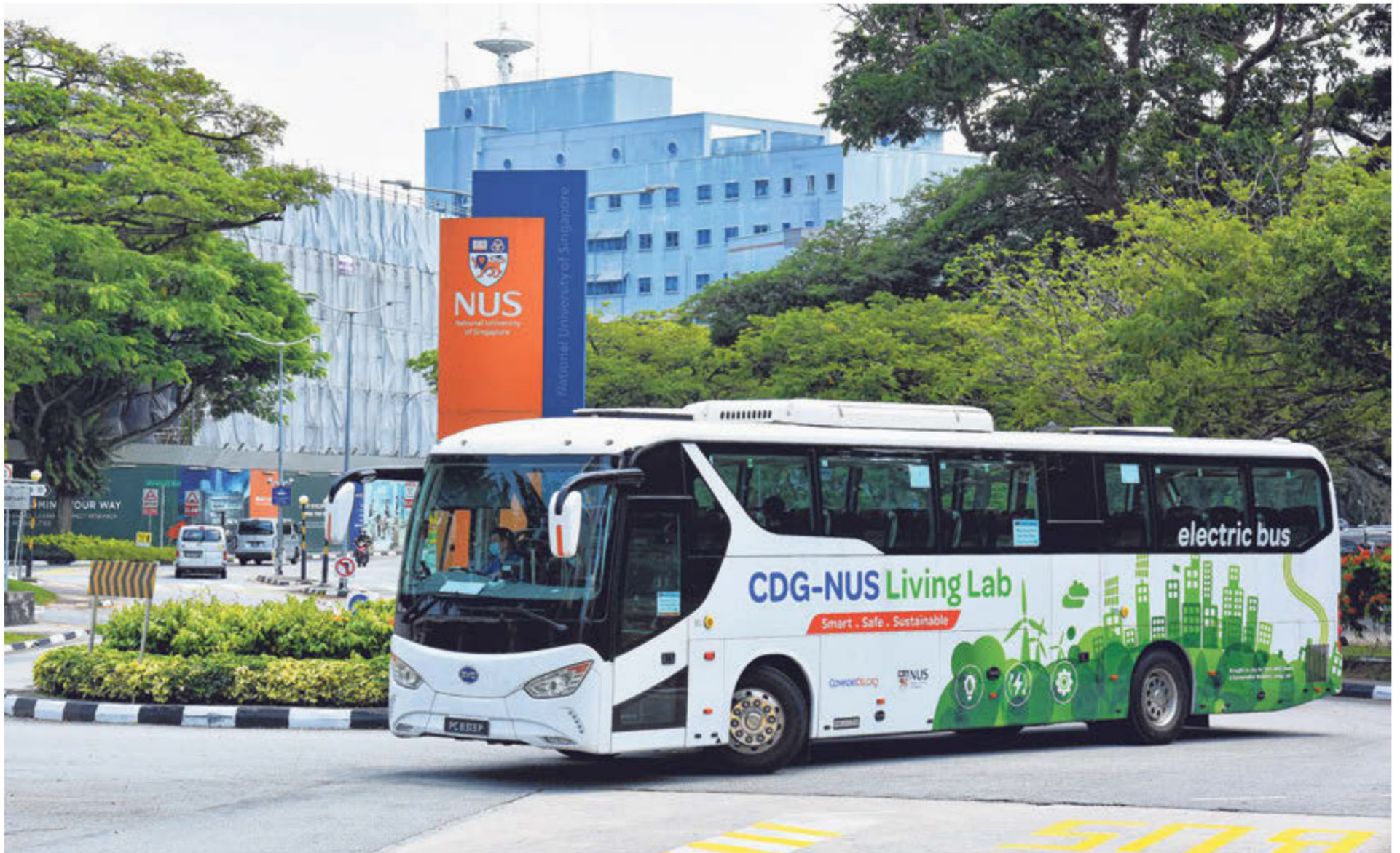
The NUS electric bus will be wheelchair accessible and equipped with smart features such as a telematics system, an anti-fatigue system as well as a forward collision and side collision warning system. PHOTO: COMFORTDELGRO
