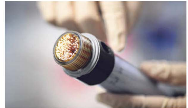
Developing membranes (above) for separating gases is far more challenging than separating liquids because gaseous particles are far smaller.
