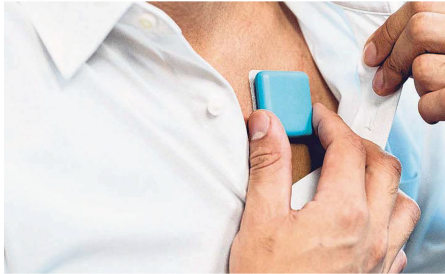
Home-grown medical start-up Respiree's wearables – one attached to the chest (left) and the other clipped over a finger – are on hospital trials to measure patients' vital parameters such as respiratory rate, breathing-pattern variability and pulse oximetry or blood oxygen level. PHOTO: RESPIREE
