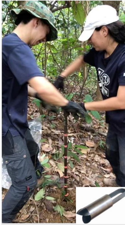
Figure 4: Soil samples were collected at every 10 cm depth intervals using a normal auger head down to 150 – 200 cm depth.
