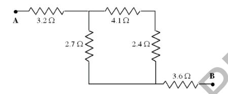
What amount of energy is dissipated in the  $2.7-\Omega$  resistor in 9.0 seconds?
