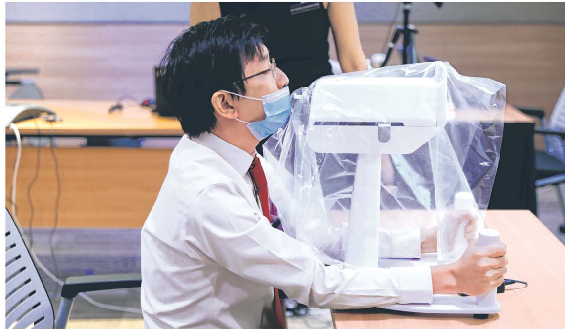
Dr Luke Tay, a consultant at SGH who was part of the team that developed the robot, demonstrating how a patient would position himself when undergoing a swab test done by the SwabBot. ST PHOTO: ONG WEE JIN
