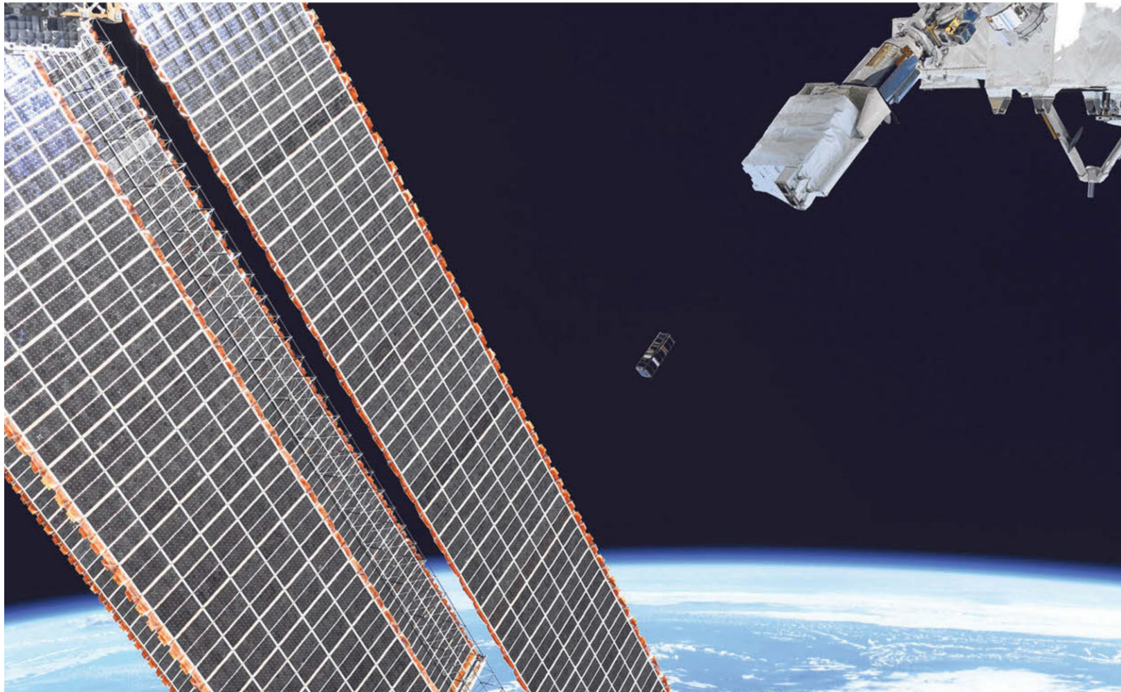
SpooQy-1 being ejected from the Japanese Small Satellite Orbital Deployer past the International Space Station's (ISS) solar arrays. This Nasa photograph was taken by an astronaut on the ISS. PHOTO: CENTRE FOR QUANTUM TECHNOLOGIES
