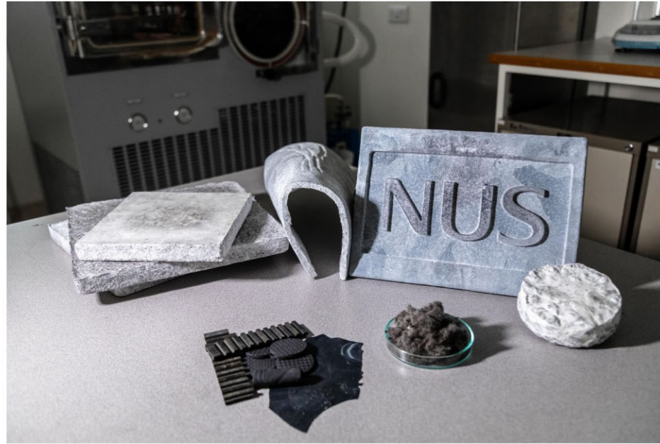
Front row: Scrap rubber and rubber fibres; Back row: Rubber aerogels in different shapes and sizes. PHOTO: NATIONAL UNIVERSITY OF SINGAPORE
