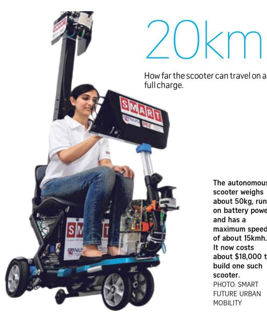
The autonomous scooter weighs about 50kg, runs on battery power and has a maximum speed of about 15kmh. It now costs about \$18,000 to build one such scooter. PHOTO: SMART **FUTURE URBAN MOBILITY**
