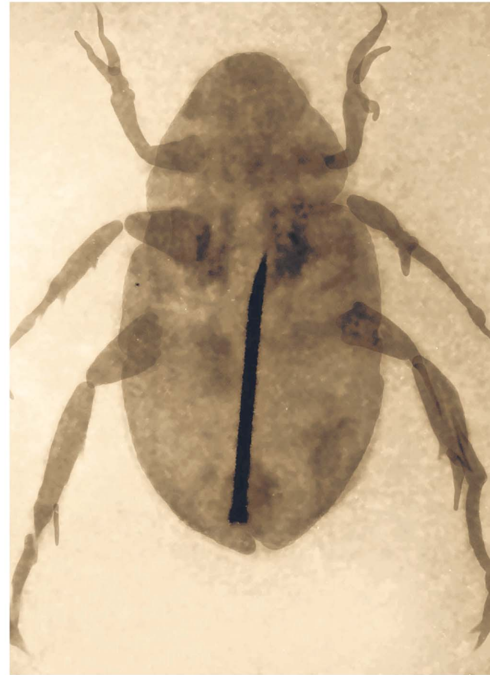
The X-ray image of the beetle specimen (left) was taken by National University of Singapore researchers using a digital camera. This was possible because the sensor they developed (above) uses nanocrystals that are thin enough for visible light to pass through.
