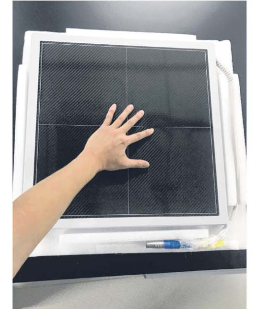
The X-ray image of the beetle specimen (left) was taken by National University of Singapore researchers using a digital camera. This was possible because the sensor they developed (above) uses nanocrystals that are thin enough for visible light to pass through.
