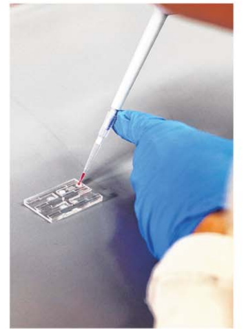
Researcher Nicholas Ho of NUS' Biomedical Institute for Global Health Research and Technology and A*Star's Institute of Molecular and Cell Biology with the enVision screening kit. For the test (right), a drop of the user's tissue or bodily fluid sample is put into a small disc. The sample then flows to another disc that changes colour from white to brown if a disease is detected. ST PHOTOS: JEREMY KWAN
