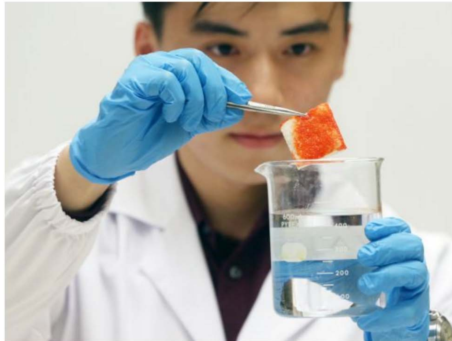
An NUS student holding a piece of cellulose aerogel used to absorb oil in a beaker of water. Photo: Ooi Boon Keong
