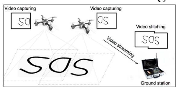
would need to be deployed to cover a large target area. The video streams from the quadcopters would be independent and disjointed, making it difficult to obtain a coherent picture. Thus, it would be helpful if the video streams were combined into a single panoramic video covering the entire target area.
