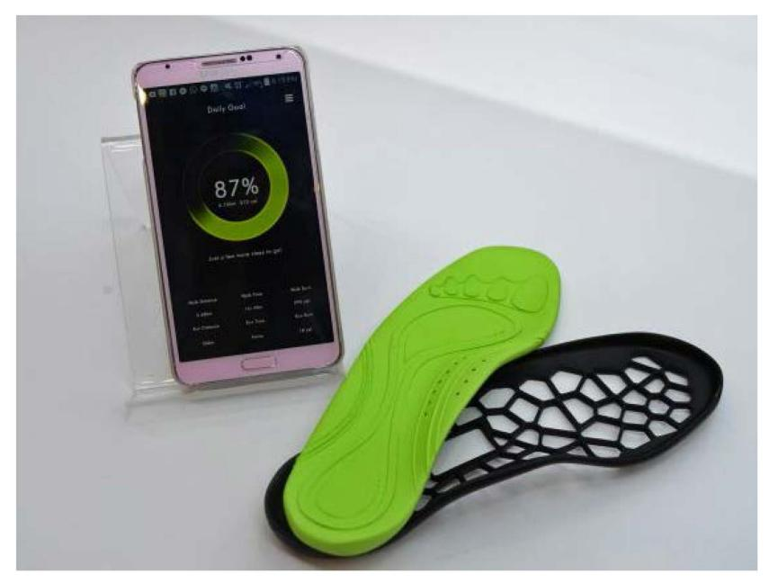
SINGAPORE — That shoe insole which is mostly used to cushion a person's foot now has a new function — to keep the foot of a diabetic patient in check through pressure sensors installed in the insole.
